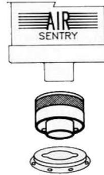
The Bayonet Adapter, Model A-104, is used to replace a standard breather cap on a hydraulic reservoir. The breather cap is removed from the breather flange on the reservoir and discarded. The adapter mounts to the flange on the tank by means of a quarter turn bayonet lug. No modification to the tank or existing breather cap flange is required.
