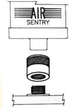
2 spin-on adapters are designed to replace the standard spin-on particle filters. These particle filters do not remove water vapor, and therefore do not protect the tank or reservoir from the worst contaminant. The adapters mount onto a male threaded pipe welded to the tank or reservoir. Model A-105 has a 1"-12 UNF straight thread and Model A-106 has a 1-1/2"-16 UNF straight thread (the 2 most common threads used in these particle filters). No modification to the tank or reservoir is required.
