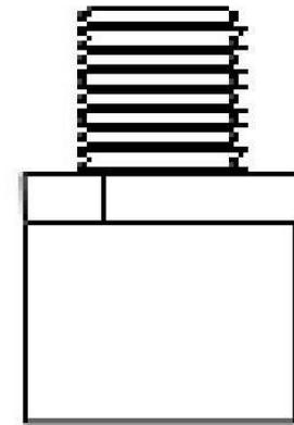
The Model A-409 adapter has a 1/2" male NPT thread on one end and a slip fit design on the other.
