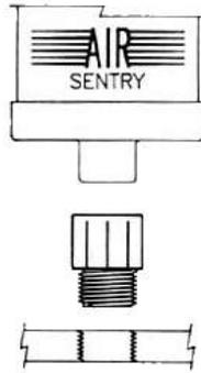
Two Threaded Adapters are intended for tanks or gearboxes with a wall thickness sufficient for a tapped hole. The thread size on the Model A-102 is 1" NPT (male) and on the Model A-103 is 3/4" NPT (male).
