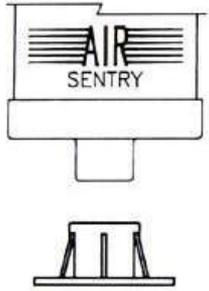
Two Flange Adapters are available for tanks where the tank wall is not thick enough for tapping threads. They are made of rugged ABS molded plastic. Model A-114 has a standard ANSI 6-hole mounting pattern, 3/16" diameter holes in a 2-7/8" diameter bolt circle. Model A-101, without mounting holes, can be drilled to match any required pattern.
